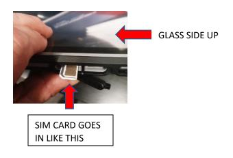
USING THE FLAT PART OF THE SCREW DRIVER , PUSH THE SIM CARD INTO THE SLOT, UNTIL IT LOCKS INTO PLACE.
