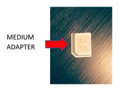
THIS IS THE DIRECTION THE SIM CARD GOES IN (METAL SIDE UP TOWARDS THE GLASS. THE FLAT SIDE OF THE SIM CARD GOES IN FIRST AND THE CUT CORNER WILL GO IN LAST AND BE ON THE LEFT-HAND SIDE. NOTE, THE GLASS SIDE OF THE TABLET IS FACING UP.
